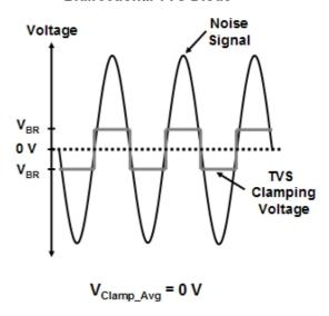
Figure 12. The average clamping voltage of a unidirectional TVS diode for a sine wave input is  $V_{BR}/2$ . The symmetrical breakdown voltages of a bidirectional device has an average clamping voltage that is biased at 0 V.
