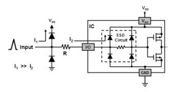
Figure 4. R forces I<sub>1</sub> >> I<sub>2</sub>, which ensures that the majority of the surge energy is diverted by the external diode array rather than by the IC's internal ESD circuit.
