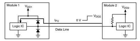
Figure 9. A diode array creates a back drive current path ( $I_{PU}$ ) to provide power through a data line when  $V_{DD2} > V_{DD1}$ .
