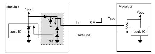
Figure 11. Back drive protection can be implemented by adding an avalanche and blocking diode to the diode array. The blocking diode eliminates the I<sub>PU1</sub> current path; however, current path I<sub>PU2</sub> will exist if the IC has a diode connected between the output and power supply pins.
