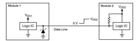
Figure 10. A TVS avalanche diode eliminates the current path (I<sub>PU</sub>) for back drive; however, the problem will still exist if module 1's logic IC uses a diode array for ESD protection.
