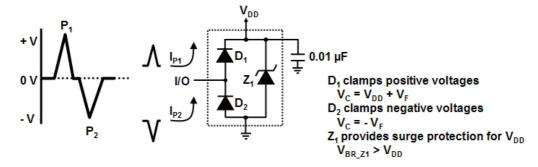
Figure 5. Adding a decoupling capacitor and avalanche TVS to a diode array enhances the ability to clamp the surge voltage to a diode drop above or below the power rails.
